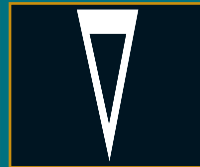
Diagram 1023B Approach to a road junction on a cycle lane where cyclists must give way to pedestrians (1875 x 625mm)
