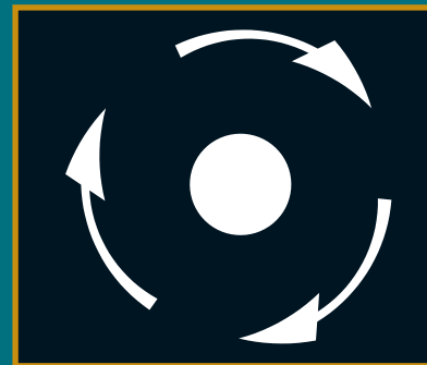
Diagram 1003.4 Roundabout 1000mm Diameter Arrows 3025mm
