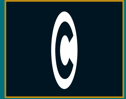
Diagram 1068 Advance warning of congestion charge (1000 x 3000mm) (1500 x 4500mm)
