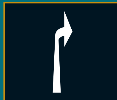
Diagram 1059 Directions in which pedal cycles should travel along a cycle lane, track or route
