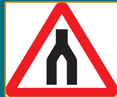
Dual carriageway road ends ahead
